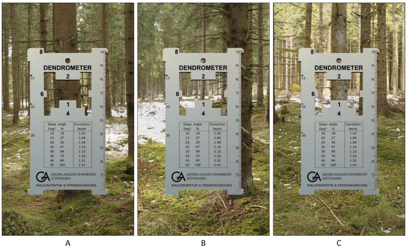
Figure 3. Angle count with BAF 1: A is a counted tree; B is outside and C is a border tree.
